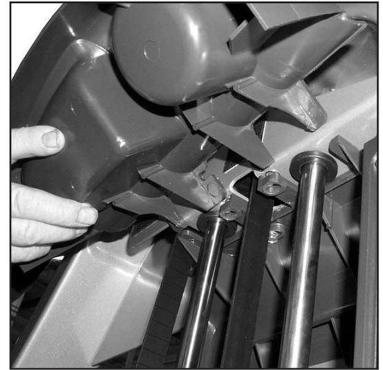
4. Remove plastic top cap by removing **front (2) bolts** from underneath shield cap with 3/8" socket.
