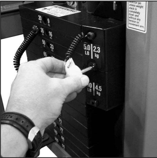
7. Insert mini weight selector pin into each mini weight to insure that the pin selects each weight with ease. The pin should insert completely into weight with no resistance. If not, adjust stand again.
