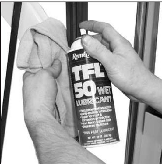
9. Lubricate only with wet Teflon spray on both the guide rods and the add-on weight guide tube. Simply wet a clean cotton cloth or paper towel. Then wipe the guide rods and guide tube down leaving a clean slightly wet looking rod or tube.
