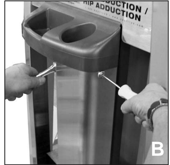
1. If the weight stack shield uses a phillips head screw and nut, remove using a phillips head screwdriver and wrench.
