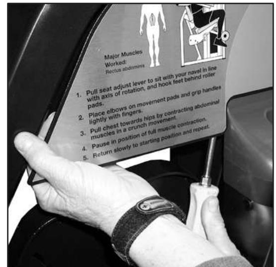
3. Insert screwdriver for leverage and remove placard shield.
