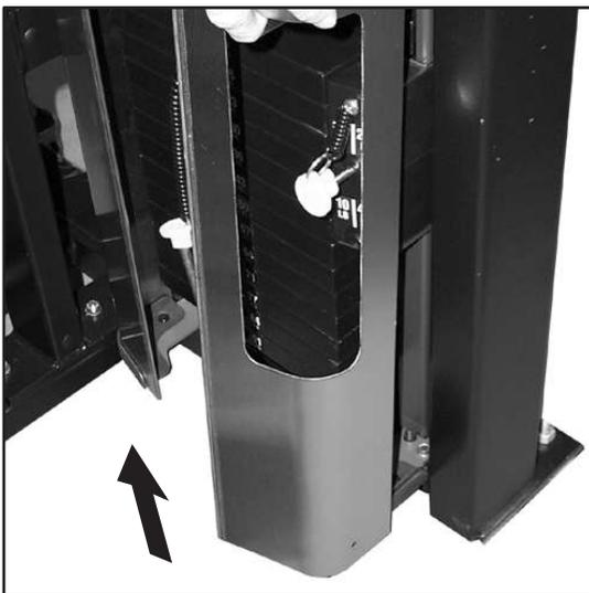
2. Lift front shields and remove from both sides.
